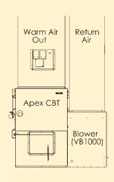
The APEX-CBT Output Plenum Size measures a large 25.75" x 24", accommodating all the hot air needed to keep you comfortable in your home. You cannot however install the APEX-CBT to where the warm air outlet operates below the height of the APEX-CBT furnace cabinet.
