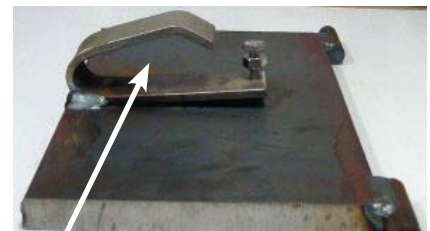
APPLY LUBE TO THE UNDER SIDE OF THE BYPASS RAMP
